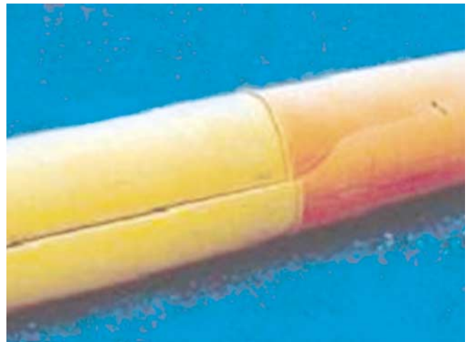
Figure 1: Arrest of a fast running fracture in PE 100
