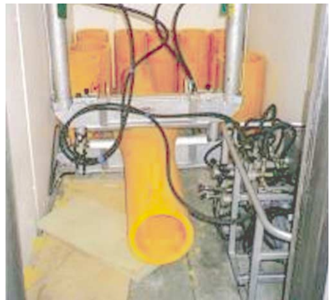
Figure 4: Squeeze off trials on PE 100 at low temperature
