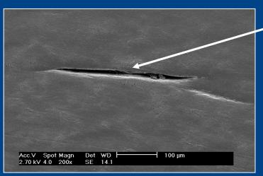
Crack starting inside the pipe
