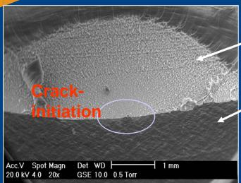
Fracture surface. The starting piont of the crack is easily seen at a macroscopic level.
