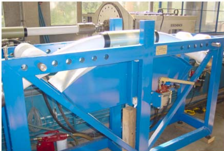
Fig.5 Bending strength test on Soluforce RTP pipe
