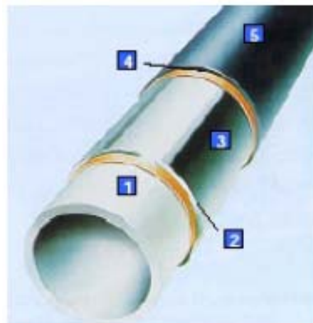
Fig. 1 Example of a typical multilayer pipe construction
