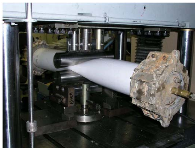
Fig.4 Squeeze-off of flexible RTP pipe
